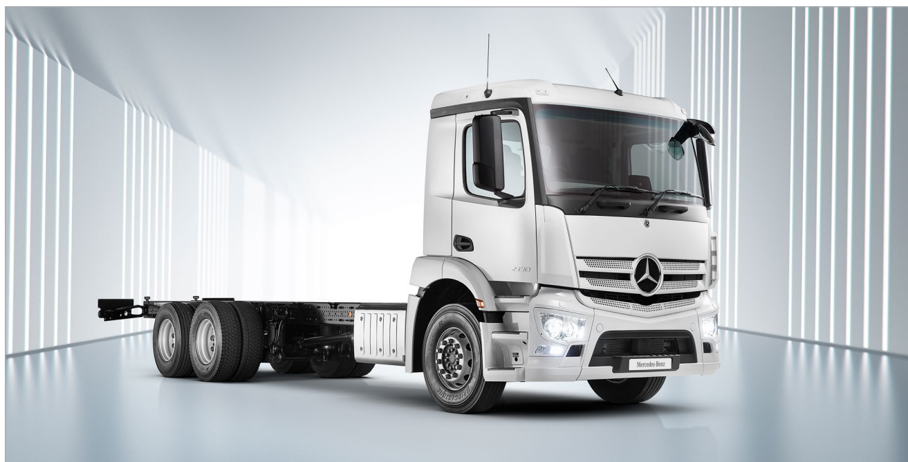
M-Cab ClassicSpace 2.30m with a 320mm engine tunnel.
